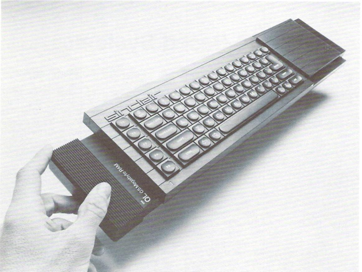
Fig. 10-1. Sinclair QL with 0.5 megabyte add-on RAM (courtesy of Sinclair).
